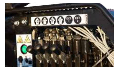
Support leg valve Electrically/manually operated. 4-6-8 sections suitable for single-circuit, dual-circuit and LS systems.
