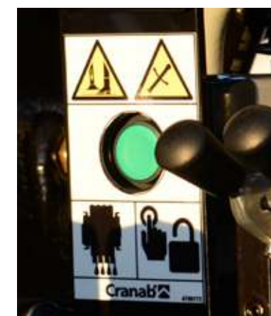
Activation lock Safety device when operating the stabiliser leg valve.
